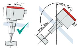
For lateral installation (horizontal shaft): Install the unit in such a way that the cable connections are on the underside of the housing.
