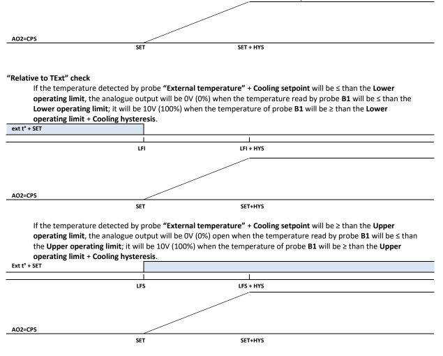
If the temperature detected by the **"External temperature"** probe + **Cooling setpoint** will be < than the **Upper operating limit** and > than the **Lower operating limit**, the analogue output will be 0V (0%) when the temperature difference detected by probes **B1** - **"External temperature"** will be  $\leq$  than the **Cooling setpoint**; it will be 10V
