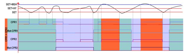
Where CPR1 / CPR2 are the statuses of compressor 1/2. Where Mot-CPR1 / Mot-CPR2 are the statuses of the timers referring to controllers 1/2.
