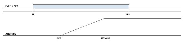
Basically, a dynamic setpoint is calculated and is equal to the sum of "External temperature" + Cooling setpoint:
