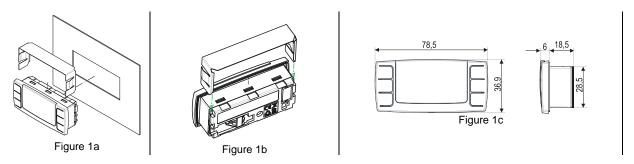
The **XW05K/XW07K** controller must be mounted by using fastening columns with a max diameter of 3.9 mm, which are inserted into the holes as specified in the next chapter.
